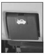
Pull the handle located inside the vehicle near the parking brake pedal.
